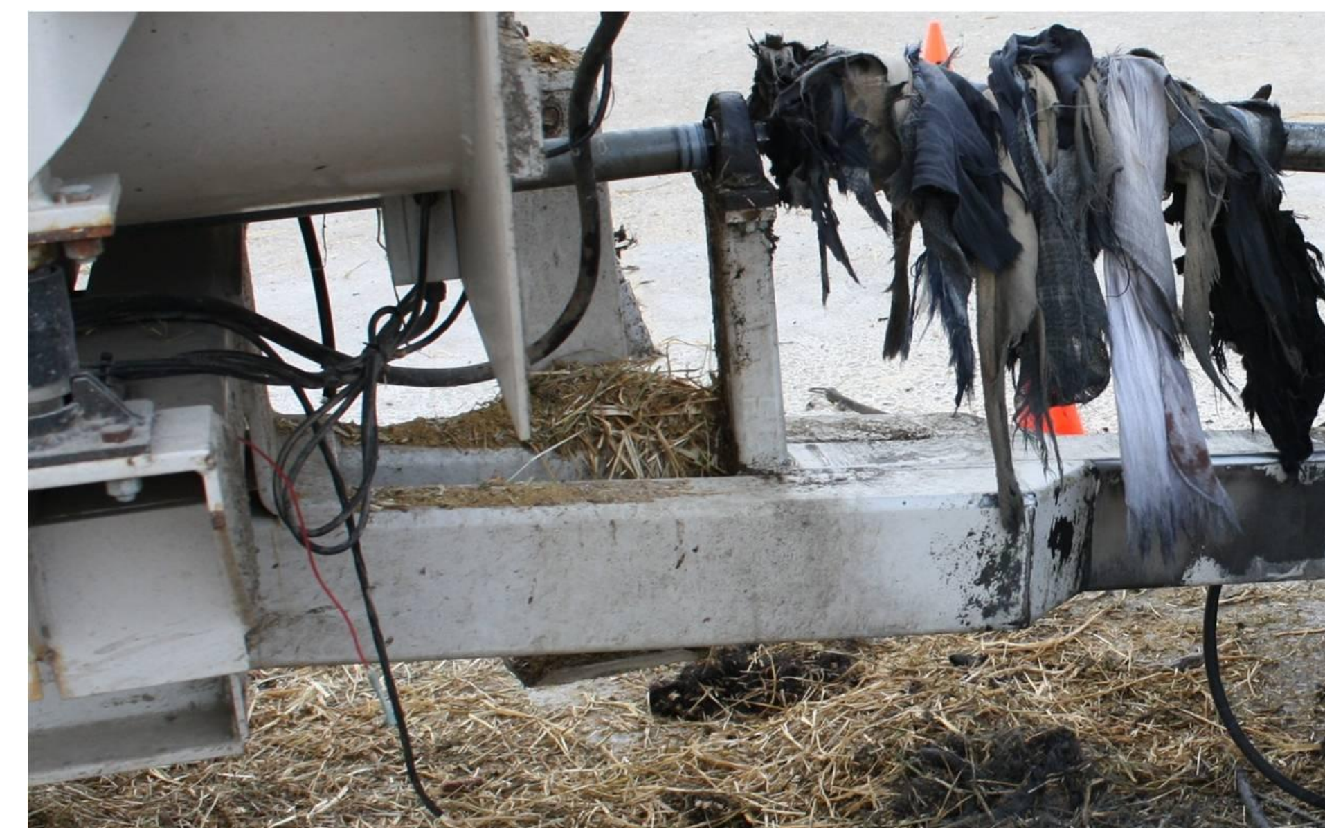
Hispanic farm hand in 20s died when shirt entangled in unguarded power take off shaft while making feed.
